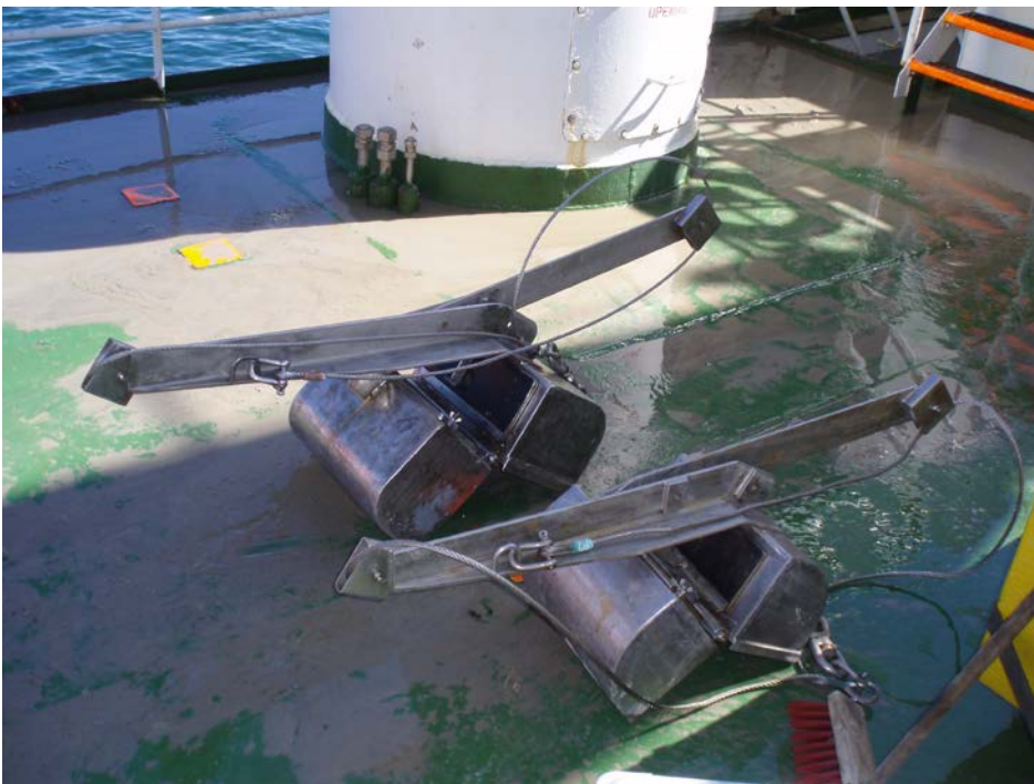
Figure 3: Combi grab of 0.15 m 2 (above) and traditional grab of 0.1 m 2 (below).
