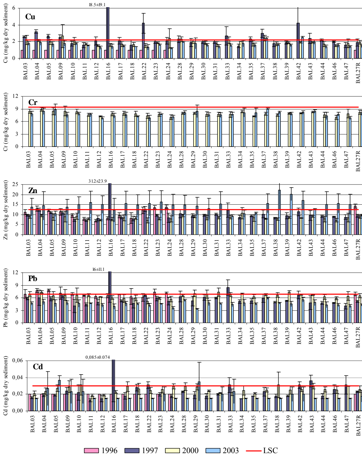
Figure 11.7. Average content and standard deviations of metals in sediment from Balder in 2003 and previous surveys. Red line is LSC central 97-03 .
