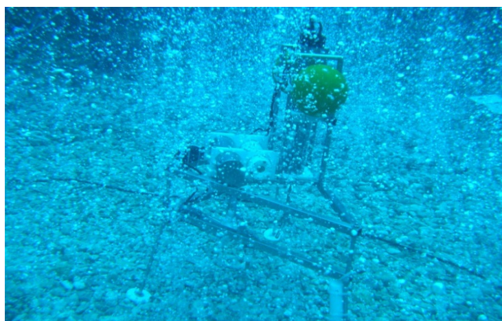
Aquatic Eddy Correlation lander deployed at Bottaro © McGinnis/PaCO 2 cruise
