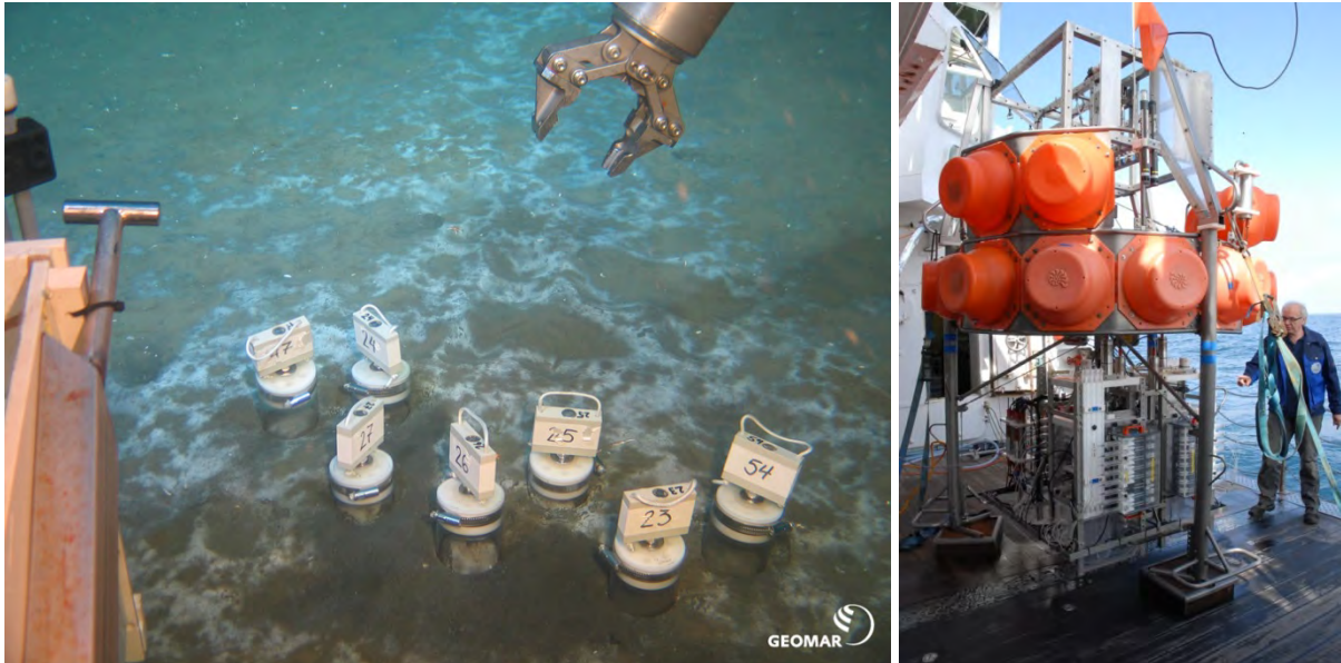
Figure 5-8: ROV Kiel 6000 is deployed at the seabed to take sediment samples from a bacterial mat patch located within the Hugin Fracture (left). Pore fluids are extracted from the retrieved sediments to determine the chemical composition and origin of formations fluids and dissolved gases seeping through the seabed. Subsequently, a benthic chamber lander is placed at the seabed (right) to measure formation water fluxes and determine emission rates (images provided by P. Linke, GEOMAR).
