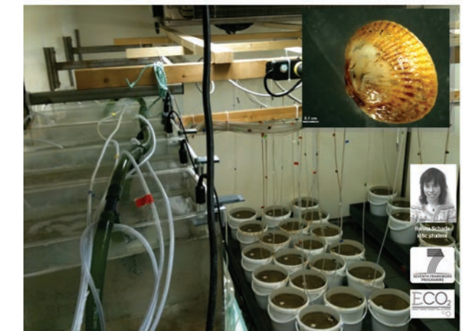
Laboratory experiments on benthic infauna bivalve communities, the bivalves show high mortalities coupled to intensive shell dissolution upon exposure to 10,000 μatm pCO 2 ; image: GEOMAR
