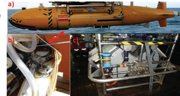
Sensors mounted on (a, b) an AUV and (c) a ROV for monitoring of pH, pCO 2 in the benthic boundary layer and water column; photos: NOC
